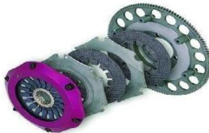
Fig: Exploded View Of Multi-Plate Clutch
