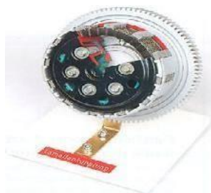
Fig: Cutaway Model Of Multi-Plate Clutch
